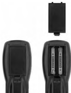
Figure 9 – Remote Battery Compartment
